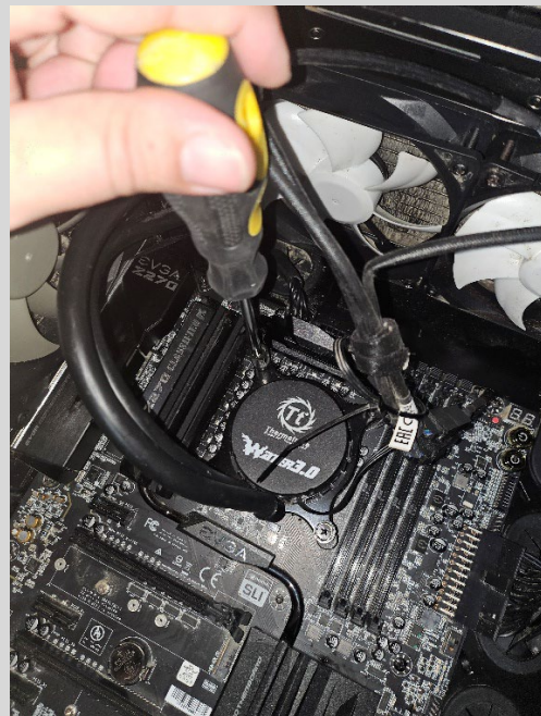
Above: attach heat sink with screws.
